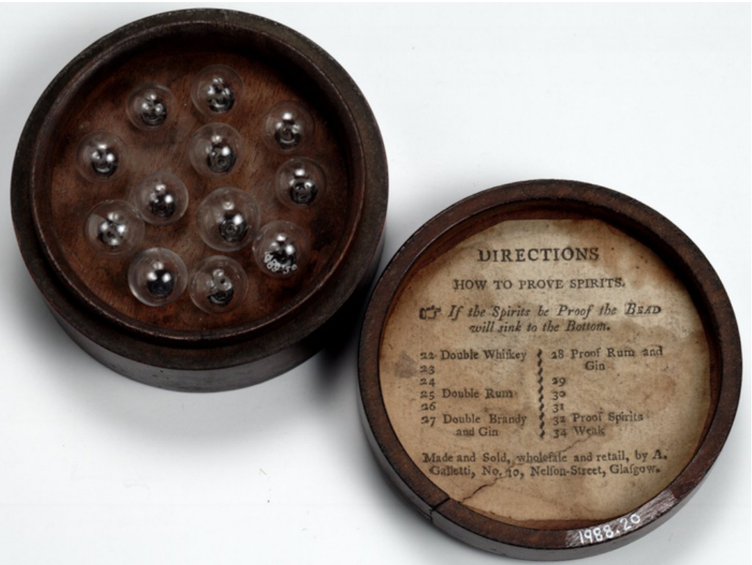
Gravity beads for measuring alcohol content, made c1805 in Glasgow by Antoni Galletti of Milan.
